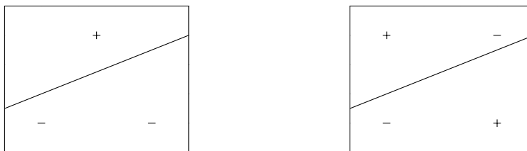
(a) Three points can always be shattered by a linear function. (b) Four points can not always be shattered by a linear function.
