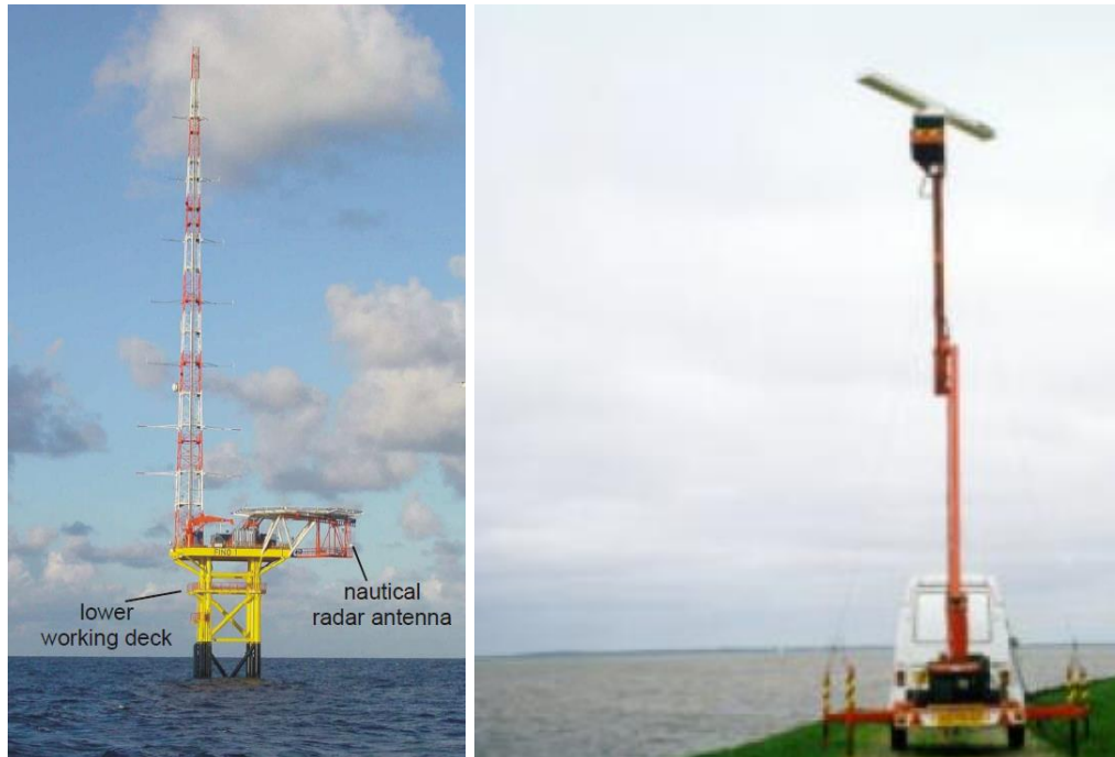
Figure 2.13. The marine radar sea surface monitoring system WAMOS II (left) (Hessner and Reichert, 2007) and SHIRA (right) (Hoekstra and Van der Vlugt, 1999).
