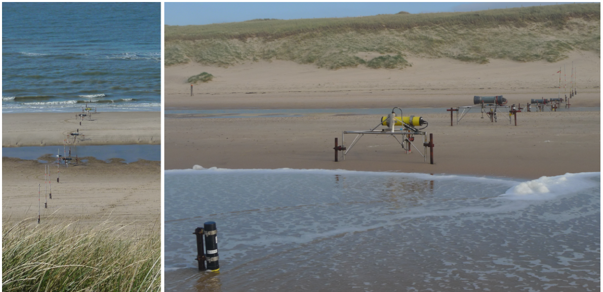
Figure 6: Overview of the cross-shore transect in seaward direction during low tide (left) and view at the instruments in shoreward direction in the last week of the field campaign, with in front a pressure gauge, followed by the tripod with ADV and one of the three mini-frames (right).
