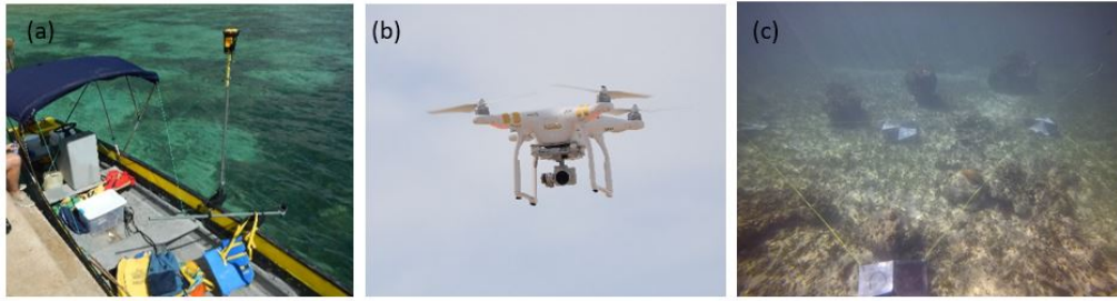
Figure 13: (a) Boat with a single beam echo sounder attached to a pole (b) Drone with a camera attached. A drone like this was used to create underwater images of the reef. (c) Ground control point at the location where the images were taken by a diver (Daly and Nienhuis, 2018)
