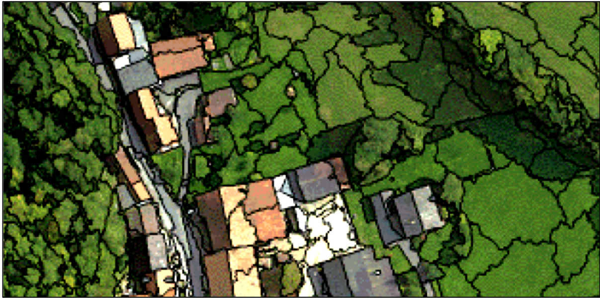
Figure 22: Example of a segmentation of with the objects being outlined in black. Note that the grassland is represented by larger objects than the trees as its pixels are more homogeneous (Baatz & Schäpe, 2000).
