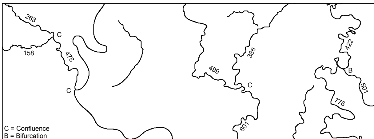
Figure 84: Subset of meander lines labelled with their calculated first order discharges (m 3 /s). Flow direction of the channels is either from west to east or from north to south.
