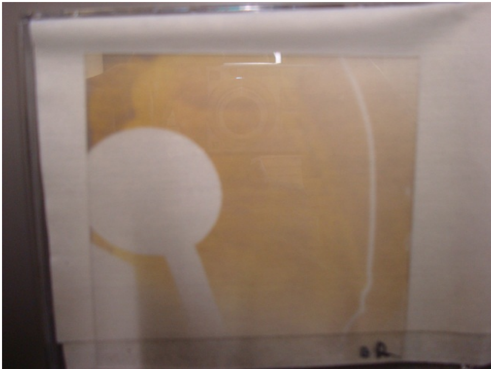
Figure 26 Glass plate after deposition to check alignment of cluster beam on substrate. The black dot represents the location of the substrate
