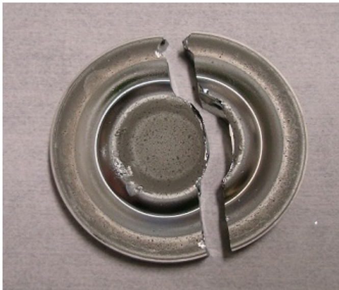
Figure 51 Broken germanium target
