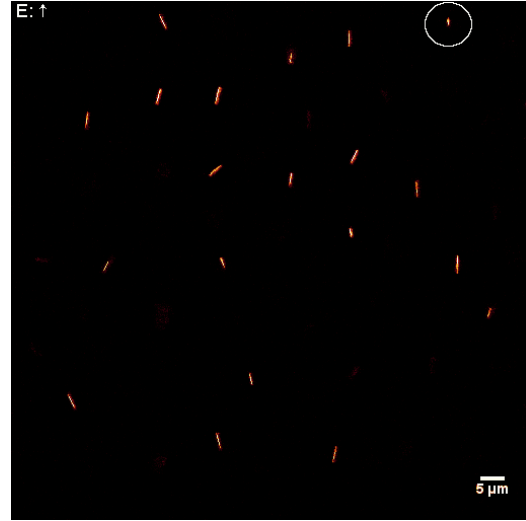
Figure 4.4: Rods (in red) and tracked rods (yellow lines) in a field of 0.045 \text{ V}/\mu\text{m}
