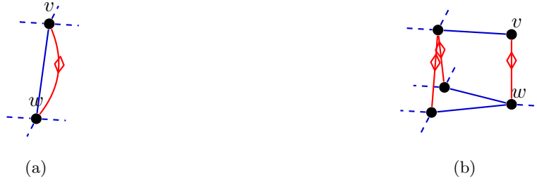
Figure 4.8: Two trivial situations considering overlaps. In (a) the edge (v \rightleftharpoons w) has to become a transfer, since v and w need to be in separate components. (b) depicts a situation where all paths from v to w are blocked by the single neighbour of v .
