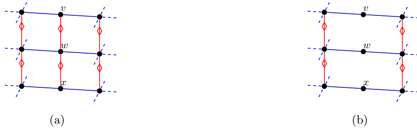
Figure 4.10: An example of when overlaps can be removed when vertices have edge degree 2.
