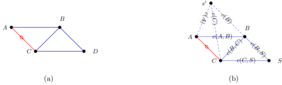
Figure 6.1: An example of how a graph needs to be modified to solve the pricing problem. In (a) the original graph is given. Subfigure (b) shows a graph where vertex D is chosen as a source and s' is added to the graph. Along the edges are the capacities of each edge, where c(b) = 1 - y_b and c(a, b) = |V|x_{a,b} .
