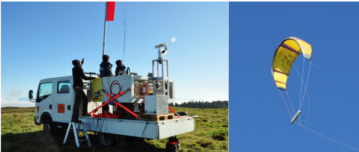
FIGURE 7-1 LEFT - FHNW KITE TEST BENCH. RIGHT - KITE AND KITE CONTROL UNIT (KCU)
