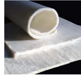
figure 6.2.2 Aerogel impregnated textile (Aspen Aerogels, 2010)
