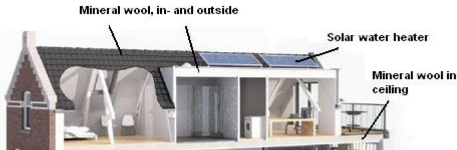
figure 3.6.2 sketch of the Sleephelling roof (Adjusted after Stichting PassiefHuis Holland, 2011)
