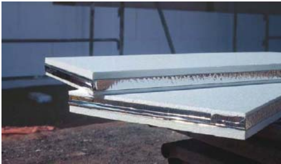
figure 6.2.6 VIP with packed in EPS (IWU, 2009)
