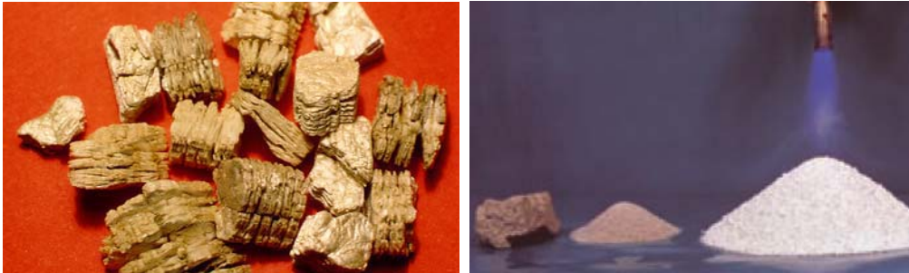
figure 3.2.5 left: exfoliated vermiculite right: expanding perlite (NVM, 2004 & Reppel, 2005)
