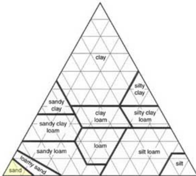
Figure 4. Diagram of loam and the soil types it consists of. Loam, in the middle of the pyramid consists of sand, clay and silt, while if there are higher concentrations of one or more of these components, the soil type can be shifted toward that corner of the soil pyramid. (Soil Characterization, 2011)
