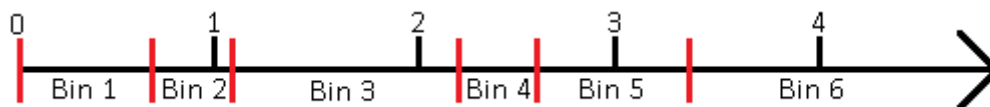
Figure 1: An example of a binning of the positive reals. With the the red lines indicating the edges of the bins. A similarity of value 1.9 will return the value of bin 2 when measured.
