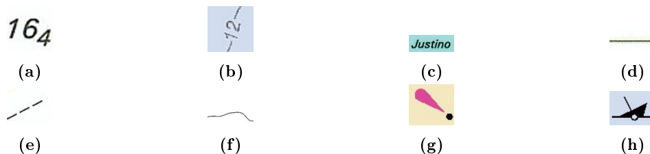
Figure 1.3. Symbols in nautical charts: a) soundings; b) depth of a contour line; c) string of characters; d) horizontal line; e) oblique lines; f) curved line; g, h) examples of other symbols.
