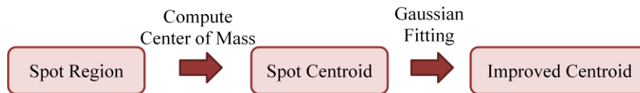
Figure 4-1-3-1 The general framework of particle localization
