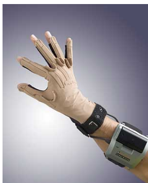
(a) The CyberGlove and its sensors.
