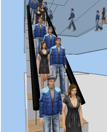
Figure 23: The zipper effect on a staircase. There is not enough space to stand side by side. This causes agents to form up in a zipper like formation. The effective use of the staircase is thus maximized.
