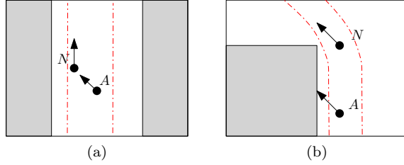
Figure 15: Problems occurring when trying to define the local stream for an agent A . The actual stream is displayed as red-dashed lines. (a) Tailing neighbouring agents leads to unnecessary collisions. (b) Following the current velocities of neighbours is also troublesome.
