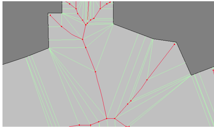
Figure 38: Edges in the Explicit Corridor Map (ECM) can vary greatly in size. Edges in the ECM are represented as red lines. (Screenshot taken in Pedestrian Dynamics)
