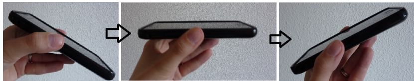
(b) Changing the moving direction into the opposite movement by changing the tilt of the mobile.
