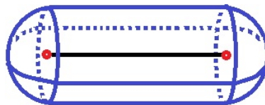
Figure 26: The bounding box of a link
