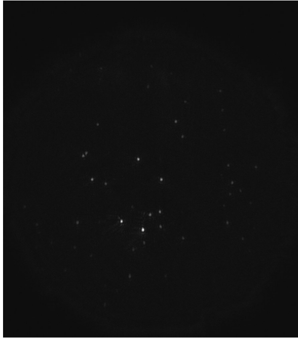
Figure 6: Microscope picture of nanoparticles. The white specks on the screen are 40 nm gold particles. The illumination is best in the middle of the picture
