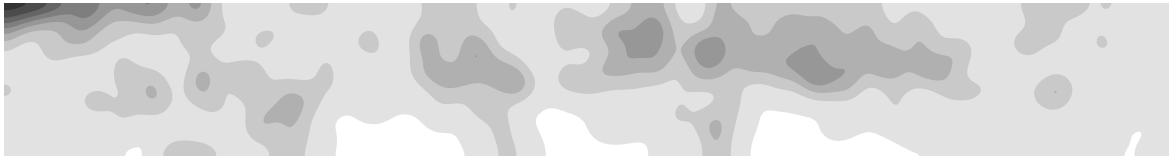
(c) Results after applying a Gaussian filter with the width of 250 pixels over image a, divided into 10 classes. The classes represent pixels values.
