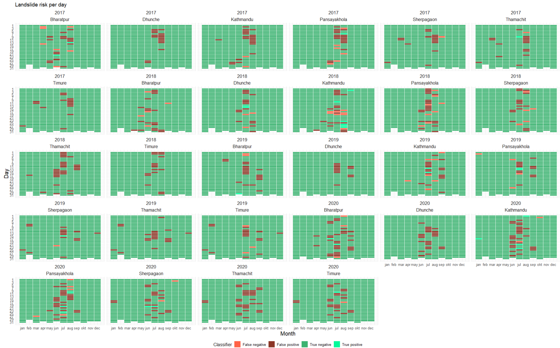
Figure C.4 Performance of ARI predicted landslide potential at Bharatpur, Dhunche, Kathmandu, Pansayakhola, Sherpagaon, Thamachit and Timure on daily scale compared to the landslide inventory of 2017-2020 (DRR Nepal).
