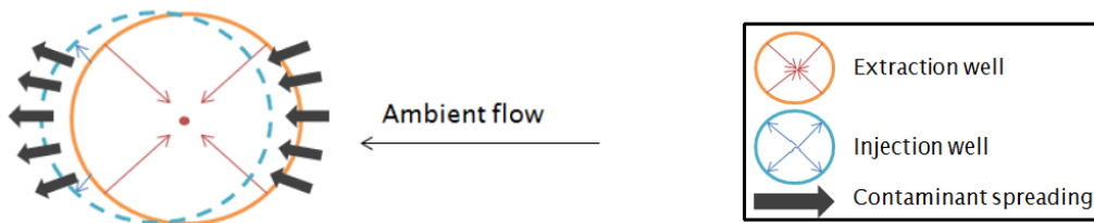
Figure 2.7 Partial recovery by ambient groundwater flow (Phernambucq, 2015).
