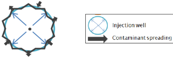
Figure 2.5 Mixing by dispersion at the boundary of the injected water volume (Phernambucq, 2015).
