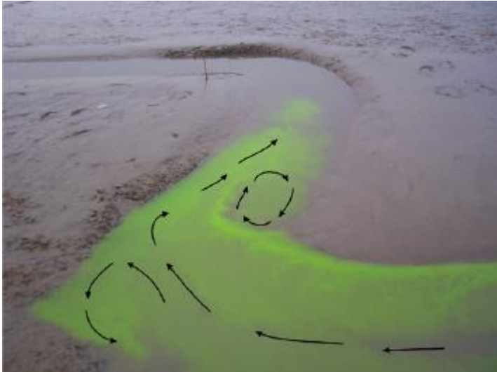
Figure 8: Flow separation in sharp bends: there are slow flowing vortices upstream of the outer bend apex and downstream of the inner bend apex (Kleinhans et al., 2009).
