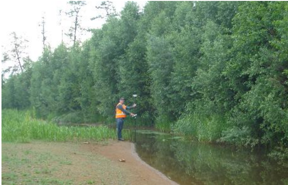
Figure 20: Measuring the waterline points by a DGPS. Notice that it is not easy to measure the waterline at the other side of the stream because of the dense vegetation.
