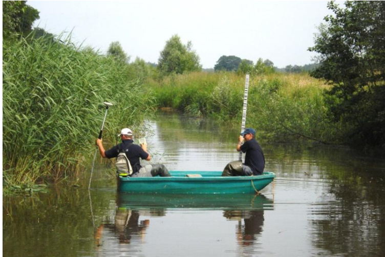
Figure 18: Measuring of profiles by RPS using a DGPS, a measuring rod and a boat (June, 2011).
