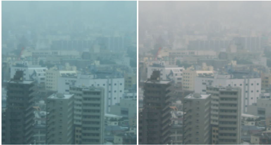
Figure 3.1: An outdoors taken photograph, due to the high colour temperature there is a bluish colour cast. After performing whitebalance the colour cast is removed.
