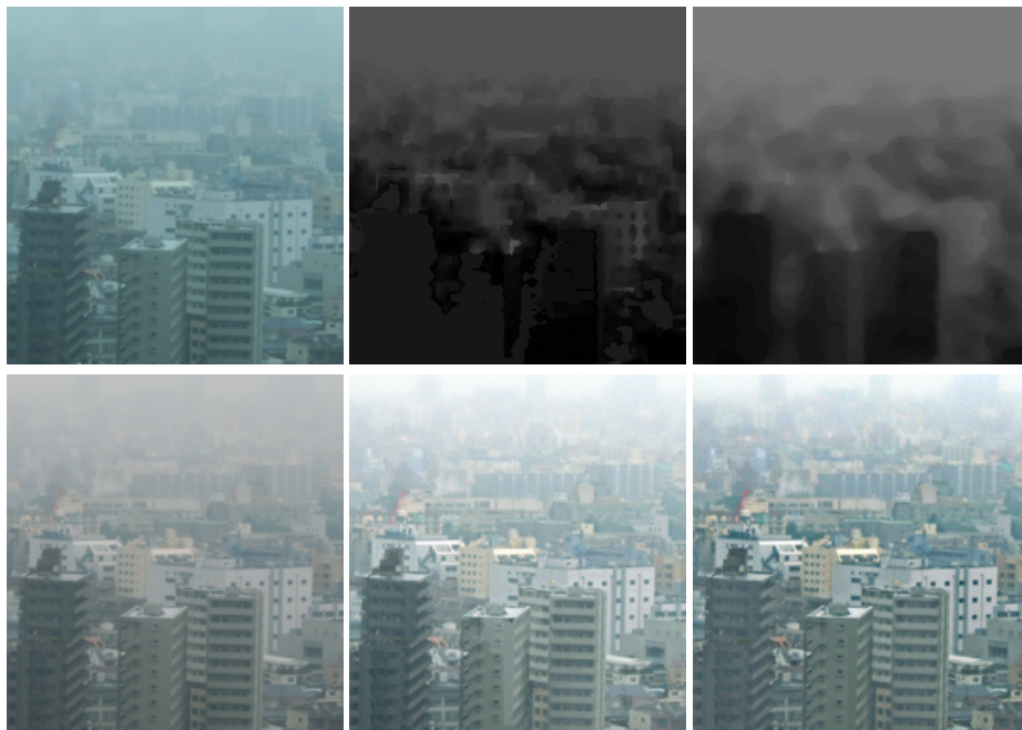
Figure 3.4: Top left: input. Bottom left: input after white balance. Top middle: airlight using MRF. Bottom middle: results using MRF. Top right: airlight using a bilateral filter. Bottom right: result using a bilateral filter.
