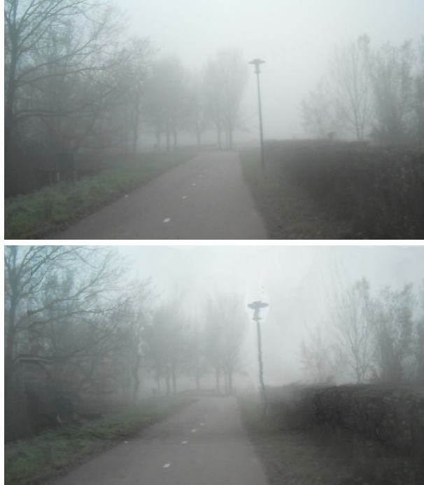
Figure 4.7: The bottom image is a re-creation of the top image which has tracked all objects for up to thirty frames and replaced the colour data of the objects with the colour data it found after tracking the objects.
