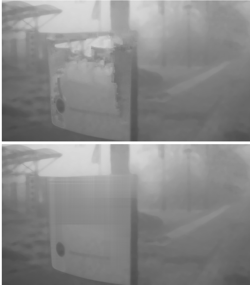
Figure 4.22: Images of which the airlight is corrected, the top image uses an inpainting algorithm while the bottom image is obtained by interpolation.
