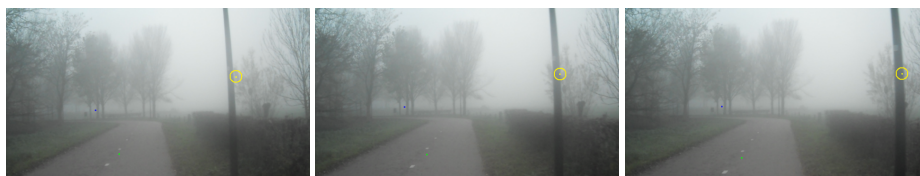
Figure 4.5: SIFT flow occlusion error. The lamppost occludes the part of the tree that is tracked and the object is lost.
