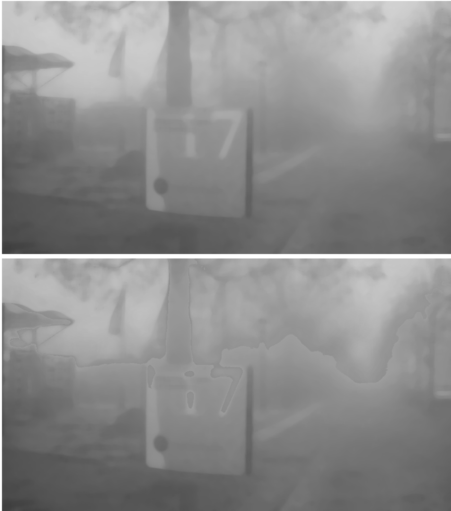
Figure 4.18: Top: Airlight of an image with a white object nearby. Bottom: Corrected airlight by deducted the depth map.
