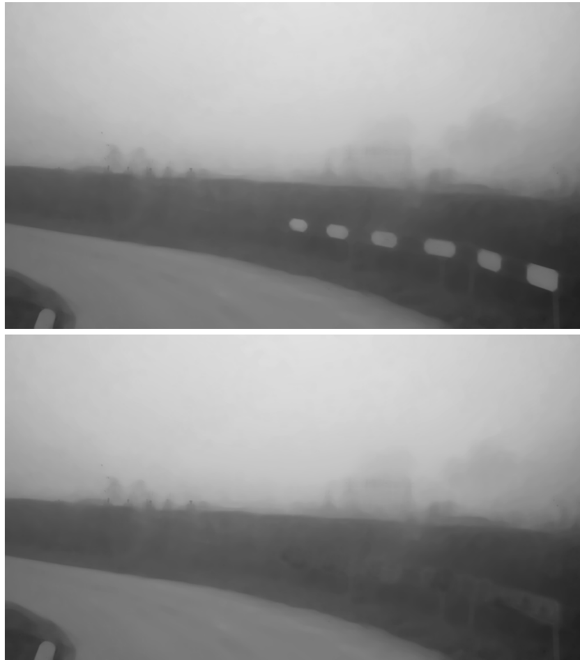
Figure 4.26: The airlight computed by Tarel et al. is shown on the top and on the bottom is the manually created ground truth.
