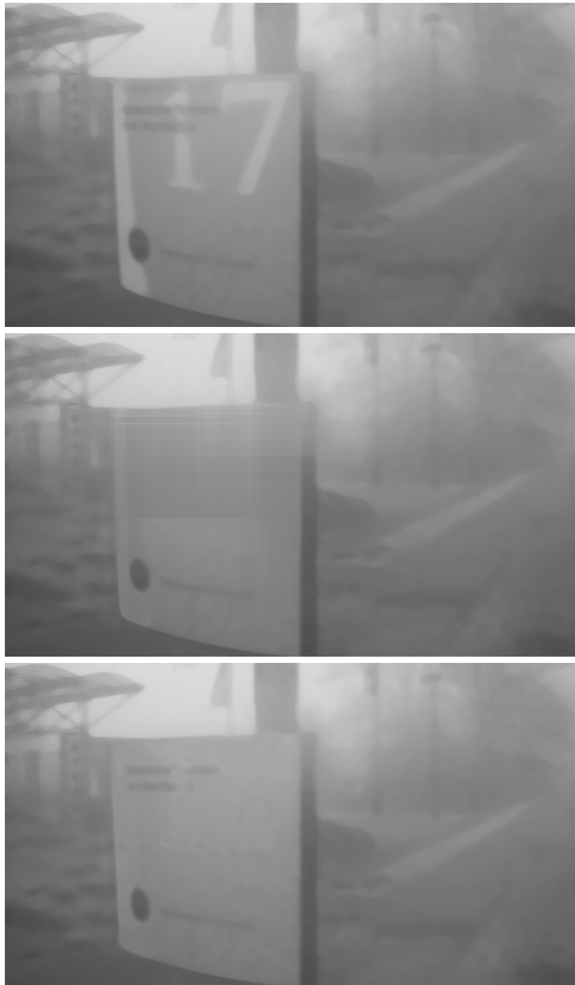
Figure 4.24: The top image is the airlight created by Tarel et al. 's method. The middle airlight image is our result, which is based on Tarel et al. 's airlight. The bottom image is the ground truth manually created using a graphics editing program. In our comparison we compare the top and middle image with the ground truth and determine the mean-error and the standard deviation.
