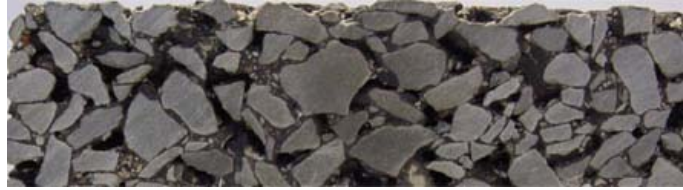
Figure 1.3: A cross-section of ZOAB which shows the stones, pockets and bitumen.
