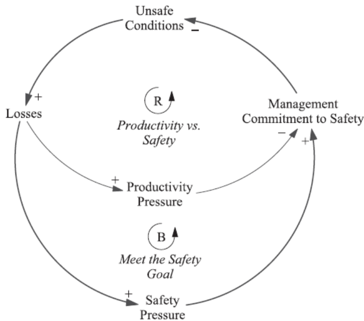
Figure 4 – Balancing productivity and safety (Cooke and Rohleder, 2006). A + means that the two variables are linked in a positive way, i.e. if one in/decreases the other does too; a – means that the two variables are linked in a negative way, i.e. if one in/decreases the other moves in the opposite direction.
