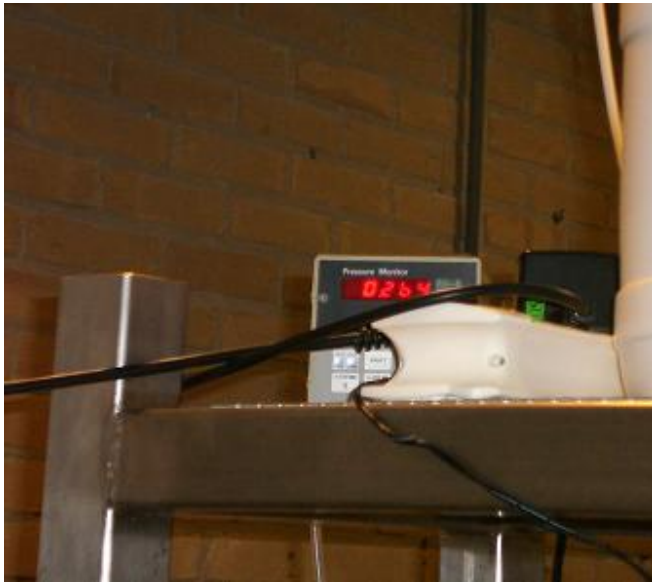
Digital pressure devise (not connected to logger), connected to Cell or Bot pressure to check the radial pressure or hydraulic head.
