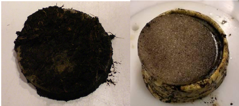
Figure 5.9: Dissection of column 4 and column 2. The figure on the right side shows filter plate of column 2 after stripping of the membrane. The figure on the left side shows the filter plate of column 4, after separation of column and filter plate. The filter plate was stuck to the peat column. By using force the filter plate could be separated from the column. A remainder of peat material was left on the filter. Between the filter and the peat material a transparent hard gel was observed.
