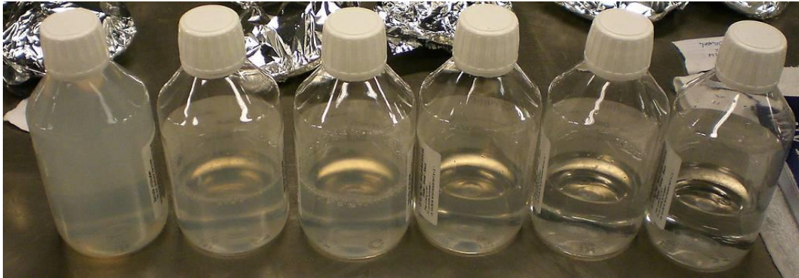
Figure 3.1: Fluid as prepared for a calibration curve at pH 7.5 prior to the retardation experiment. Initial concentrations from left to right: 1981 ppm \text{SiO}_2 / ppm L200, 1238 \text{SiO}_2 / ppm L200, 945 \text{SiO}_2 / ppm L200, 546 \text{SiO}_2 / ppm L200, 297 \text{SiO}_2 / ppm L200 and 20 \text{SiO}_2 / ppm L200 ppm L200.
