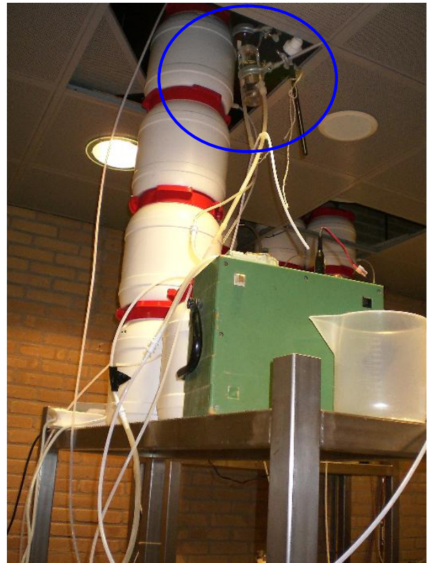
Small storage flask, creating the hydraulic head during reactive tracer infiltration.
