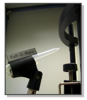
**Figure 1:** *The hard-plastic tip at the end of the air puff apparatus.*
