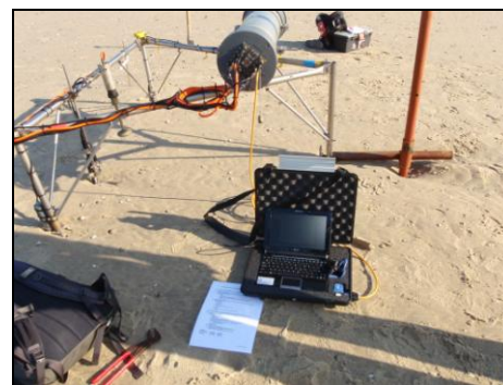
Photo 3-2: a: Tripod with EMF, OBS, pressure sensor and data logger, b: COM-port connection with laptop.
