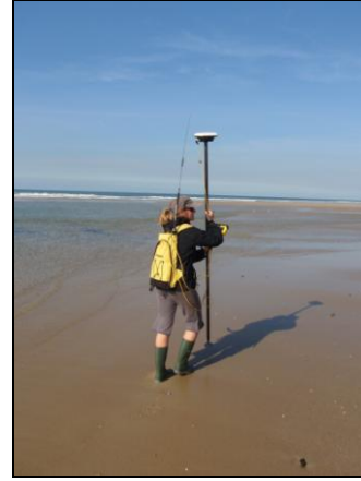
Photo 3-4: a: DGPS base station with radio on the left and receiver on the right, b: Mobile DGPS device.
