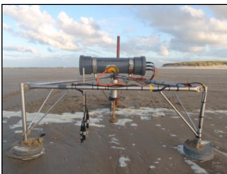
Photo 3-2: a: Tripod with EMF, OBS, pressure sensor and data logger, b: COM-port connection with laptop.
