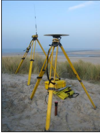
Photo 3-4: a: DGPS base station with radio on the left and receiver on the right, b: Mobile DGPS device.
