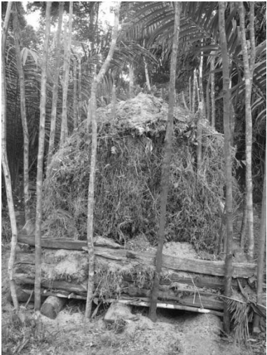
Image 5.5 The traditional way of making charcoal: piles of logs and branches are covered by sand, leaves and moss and burned slowly to carbonize - Alloakpoke
